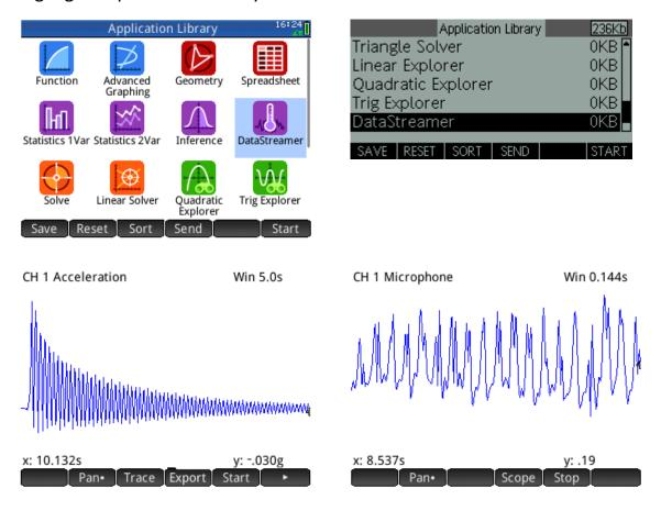
There are a variety of probes which can be used. The first example above show the output when an acceleration probe is attached to end of a steel rule held firmly on the edge of a table and 'twanged'. The second example is the output from blowing into a microphone.
